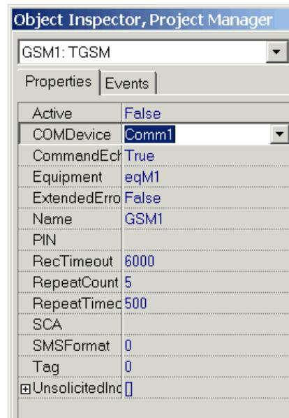
*TGSM* component must be active to work. Call *GSM1.Open* method or set *GSM1.Active=True*. Component establishes communication with a GSM module.
